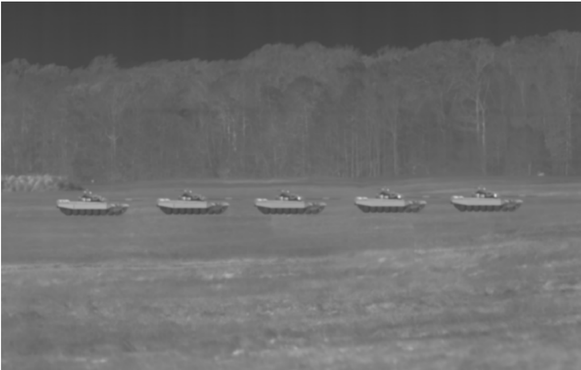
Figure 6: Rendered MBTs, from left to right, first is physical temperatures, second is diffuse approximation in MuSES, third is rendered diffuse, fourth is the Sandford Robertson standard coating, and the fifth is a standard coating with a more narrow specular lobe.
